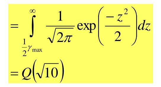
From the table of Gaussian probabilities ,we<sup>\*</sup> get P<sub>e</sub>  $\bigoplus$  0008 and Average error rate  $\bigoplus$  p<sub>e</sub>/sec = 4 bits/sec
