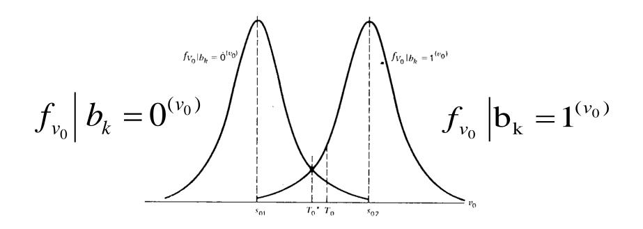
:The optimum value of the threshold To\* is\*
