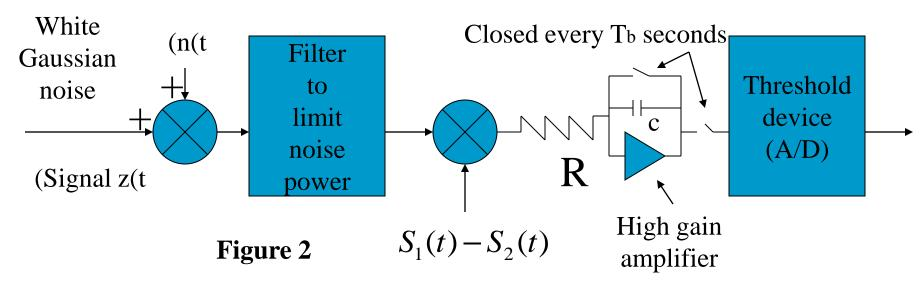
The bandwidth of the filter preceding the integrator is assumed \* !!! to be wide enough to pass z(t) without distortion 2 **Example:** A band pass data transmission scheme uses a PSK signaling scheme with
